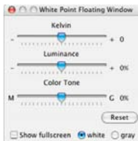
The Whitepoint Editor allows to adjust the whitepoint for a screen to screen or screen to viewing booth match.
