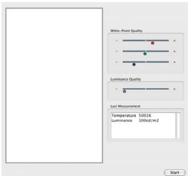
Quality indicators help adjusting the display close to the target.
